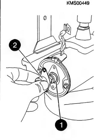
Checking armature braking torque
